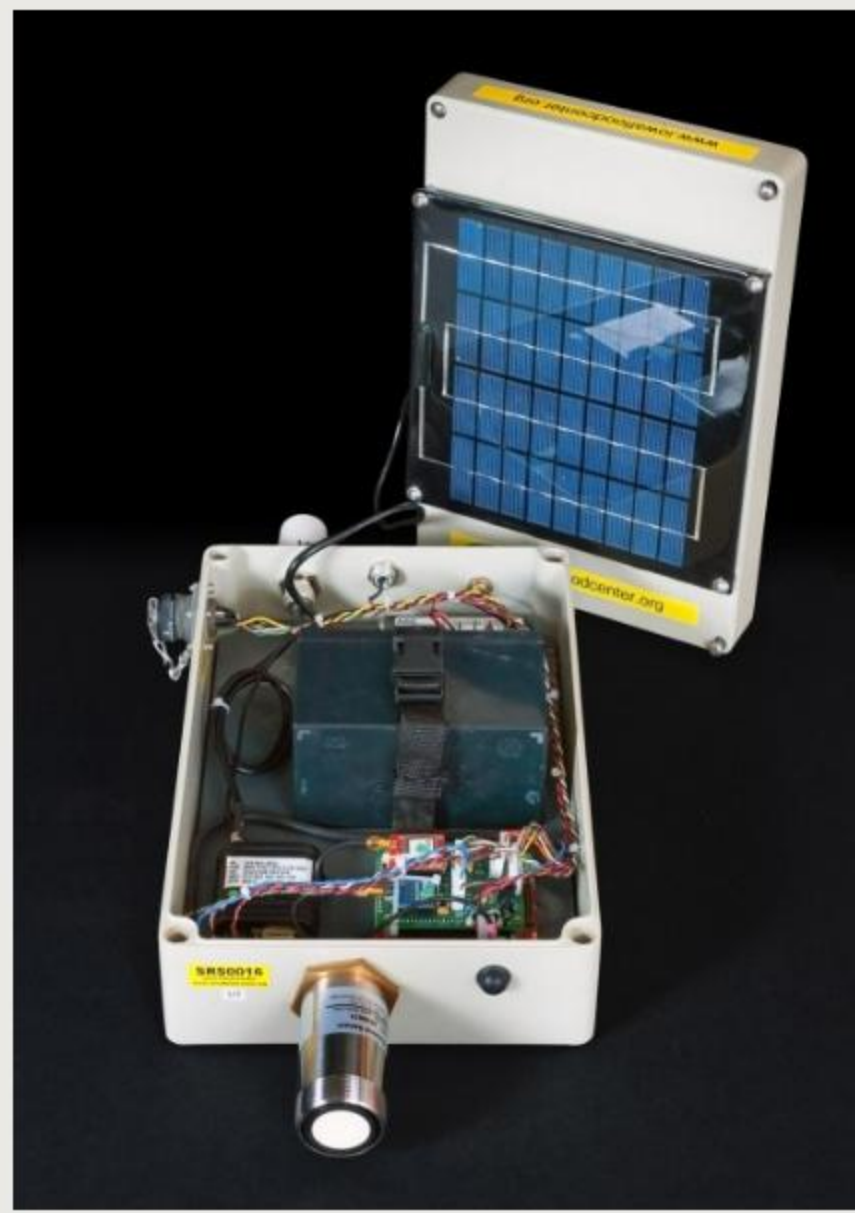
One of the Iowa Flood Center's priorities has been to create an affordable stream sensor.
