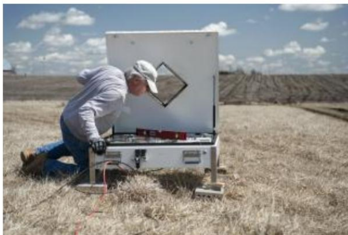
Two-dimensional video disdrometers (2DVDs) will measure size, shape, speed, and number of raindrops. Photo by Aneta Goska, Iowa Flood Center.
